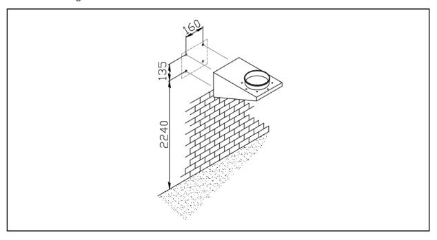
The wall console is principally required for all telescope arms that are to be fastened to the wall. The wall console is used as a connecting point for the downstream extraction.
